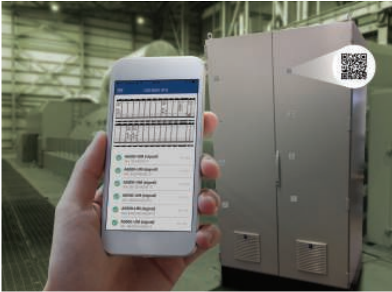
FIGURE 2. The ATG View application provides mobile access to critical asset health information from Emerson's CSI 6500 ATG machinery protection and prediction monitoring system. Users can scan a quick-response code located on the cabinet and view the status and health of all cards and measurements from the associated rack on their mobile device
