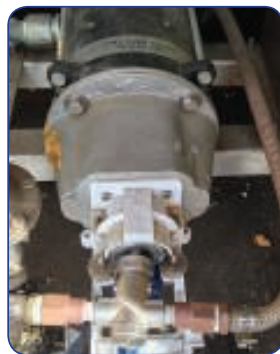
The QDX pump doses methanol with no danger of losing prime
