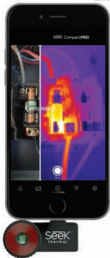
FIGURE 3. The CompactPRO plugs directly into a smartphone device, giving the user instant connect-and-detect convenience and versatility, turning the smartphone into a thermal-imaging camera and combining it with an app that maximizes heat-sensing technologies to prevent damage, increase productivity and visually image the necessary details within heat signatures
