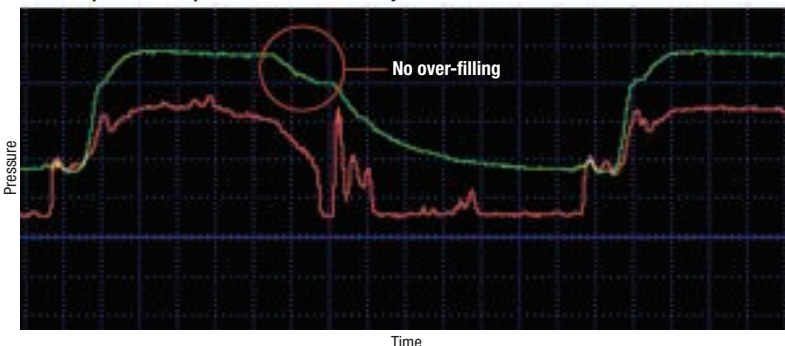
FIGURE 3. Some AODDs experience wasted air when overfilling occurs at the end of each pump stroke, but modernized air-distribution systems allow for more optimized air consumption by eliminating overflow
