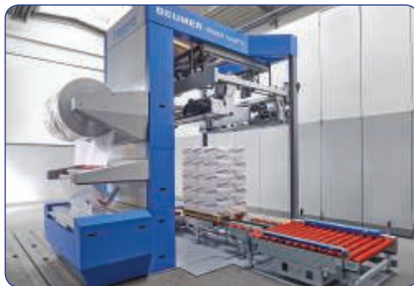
Stretch hood packaging equipment gives extra protection for palletized goods during storage and transport
