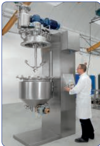
The EKATO SOLIDMIX VPT removes solvent that is beyond the reach of spray dryers
