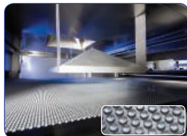
The Rotoform system yields uniform, free-flowing pastilles from melts with viscosities up to 40,000 mPas
