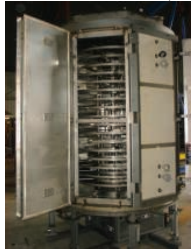
FIGURE 2: The stacked, circular trays of the Turbo Dryer have been used for several applications in drying recycled material
